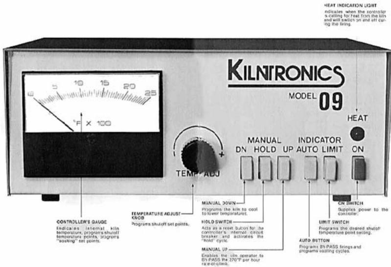
Refer to the front panel of your Temperature/Rate Controller as you read through the following explanation of what each front panel feature is and does. Don't be afraid to push the buttons and turn the knob. You won't break anything.
